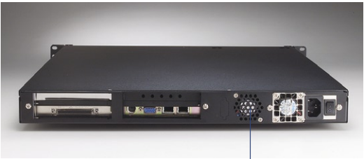
One 10-CFM cooling fan is on rear-end
