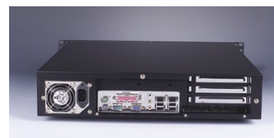
300W ATX PFC P/S & rear panel of motherboard version
