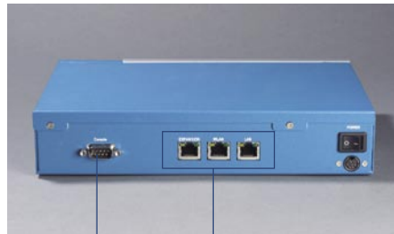
RS-232 console port Three LAN ports
