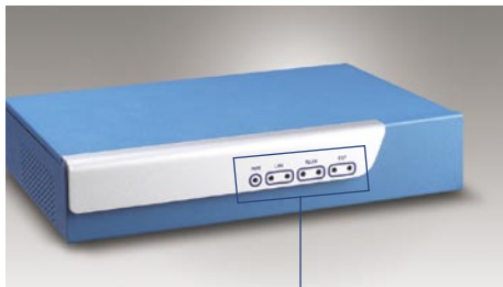
Seven LED indicators (Power x 1, LAN x 3)
