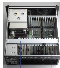
Hold-down clamp Max. 14-slot backplane
